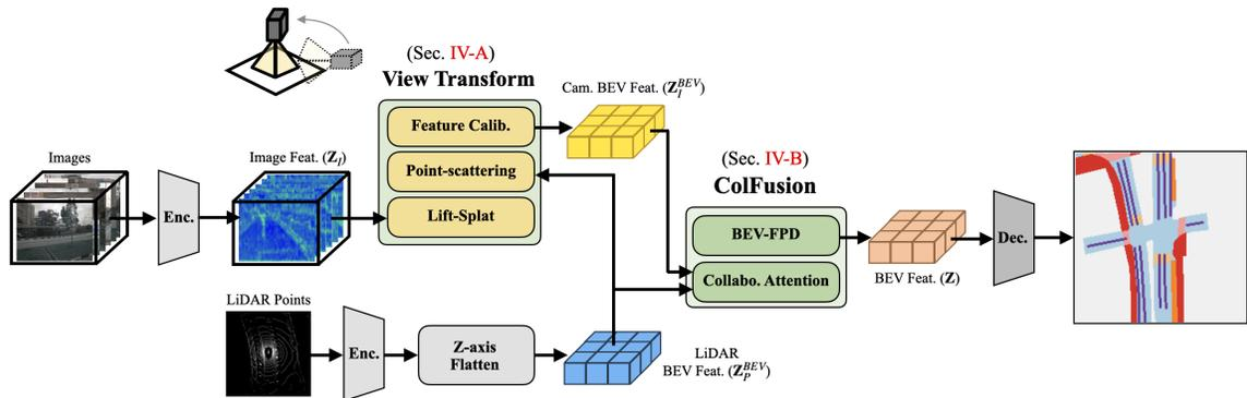
Fig. 2: **Overall Scheme of BroadBEV.** Our view transform takes in LiDAR BEV feature ( $\mathbf{Z}_P^{BEV}$ ) to lift and splat [31] image features ( $\mathbf{Z}_I$ ) with our proposed Point-scattering to camera depth distribution. Then it calibrates the camera BEV feature. After preparing camera and LiDAR BEV features, ColFusion which consists of collaborative attention and BEV-FPD [42] fuses them into a unified BEV feature ( $\mathbf{Z}$ ). BroadBEV decodes the feature into a constructed map.
