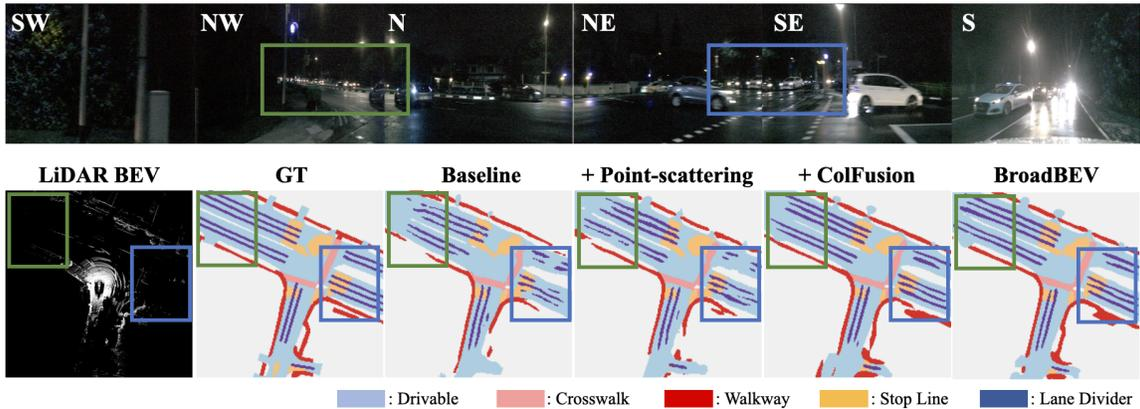
Fig. 7: **Ablation Study on Broadness.** The upper row displays RGB images. The lower row contains LiDAR BEV and map construction of our variated models. “**Baseline**”, “**+ Point-scattering**”, and “**+ ColFusion**” respectively correspond to “Baseline”, “w/ Scat.”, and “w/ Fusion” models in Table IV. Green ROIs show Point-scattering’s contribution to broad-sighted perception. Blue ROIs demonstrate ColFusion’s enhancement of perception performance in distant regions.
