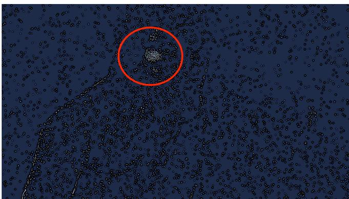
Fig. 3. Screen-grab from Metavision Studio rendering of event camera recording of a subject's wrist. The placement of the coloured dot on the wrist can be seen in the top right part of the image as a cluster of white dots.
