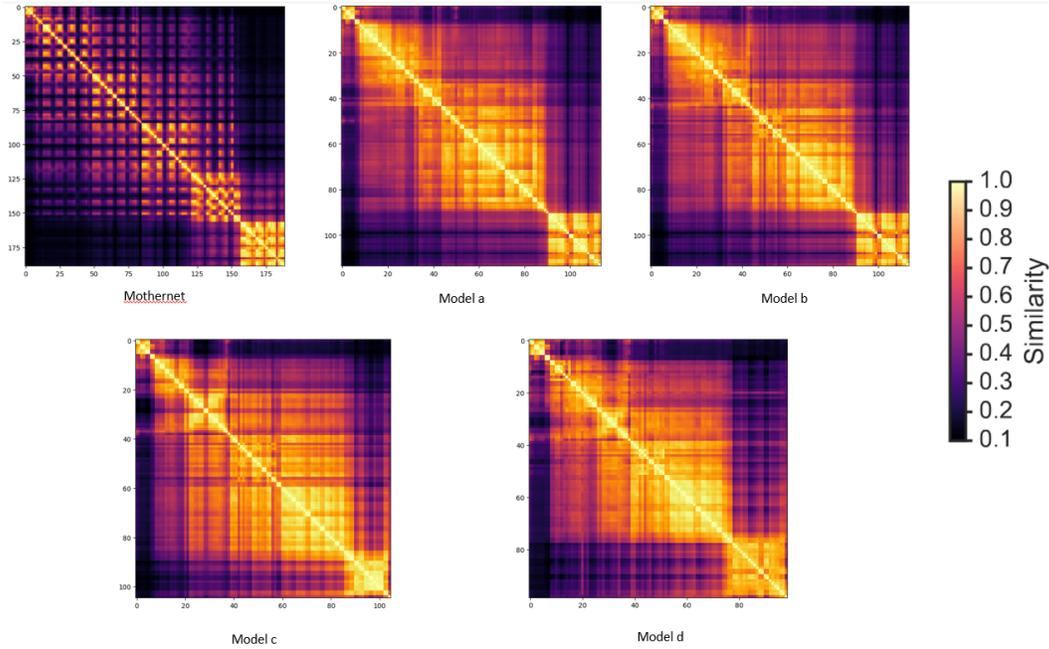
Figure 4: Here, the Mothernet has checkerboard heat map displaying local similarity and model learns different representations across layers. The compressed models (Model a, Model b, Model c and Model d) demonstrate progressively increasing similarity across multiple layers. This suggests that Model a is the best-compressed model in terms of learning distinct representations across layers. This correlates with the performance of the trained model as well as the surrogate loss used in this work.
