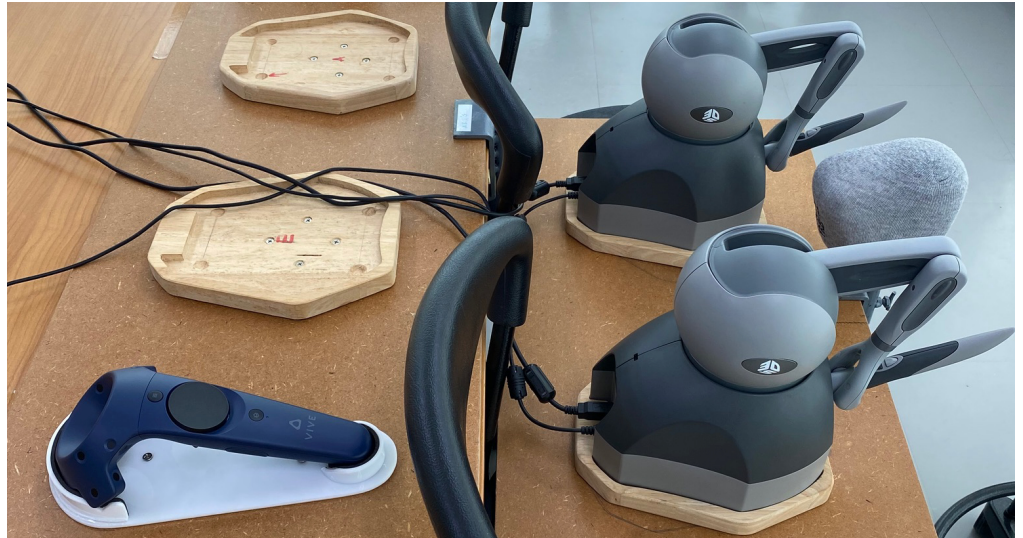
Fig 3. The calibration of the haptic devices with the HTC Vive VR system is implemented using a VR controller with a static offset. The "hand-tool misalignment" is achieved by calibrating and then moving the haptic devices forward and downward in front of the table, as shown here. Republished from [27] under a CC BY license, with permission from IEEE, original copyright 2022.
