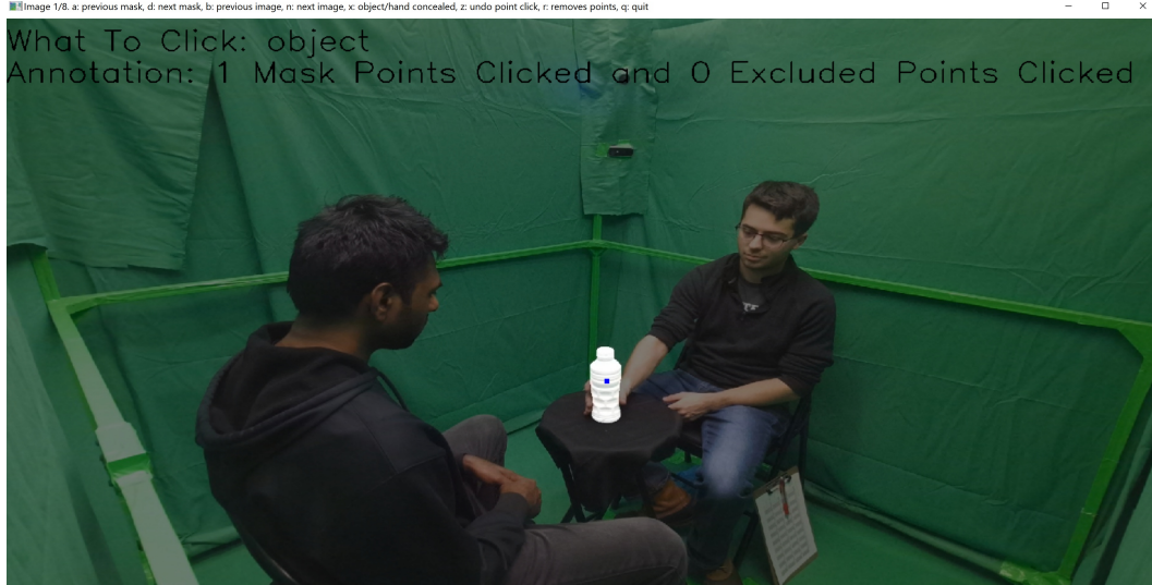
Figure 11: The annotation tool for selecting masks from the full image segmentation. Inputs are mouse clicks and keypresses which correspond to mask selection and saving, respectively.
