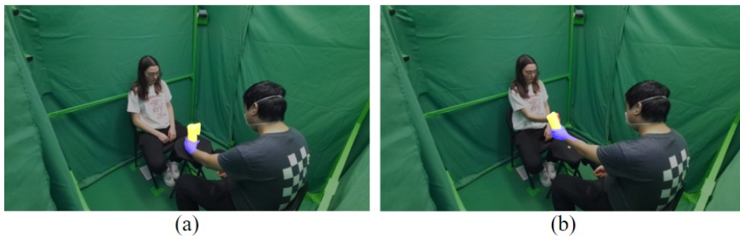
Figure 13: Hand and object mask tracking with the giver's hand in blue, the object in yellow, and the receiver's hand in red. The giver hand mask is increasing up the giver's arm from (a) Frame G, to (b) Frame T.
