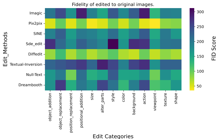
Figure 14: FID Heusel et al. (2017) score computed between the original images and the edited images across all the 8 methods tested on EDITVAL. Lower FID score quantitatively indicates a better image quality. We calculate FID score by computing Fréchet distance between two Gaussians fitted on the set of original and edited images. By default, Heusel et al. (2017) works with the final layer features from Inception network, but, due to limited samples, we can use a shallow feature-layer even though the FID score may no longer reflect the visual quality accurately.
