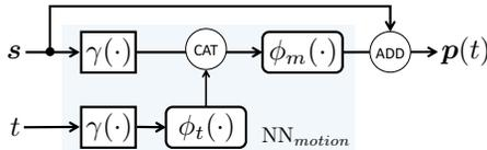
Figure 4: Computational structure for time-varying position of a particle.  $\gamma$  is the positional encoding function (Mildenhall et al. 2020),  $\phi_m$  and  $\phi_t$  are 3 and 2-layer MLP, ‘CAT’ is concatenate operation and ‘ADD’ is element-wise addition.
