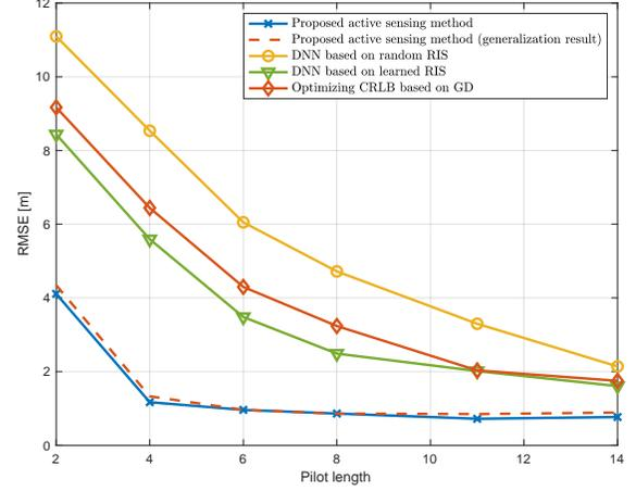
Fig. 4: Localization accuracy vs. pilot length,  $N = 64$ , SNR= 20dB.
