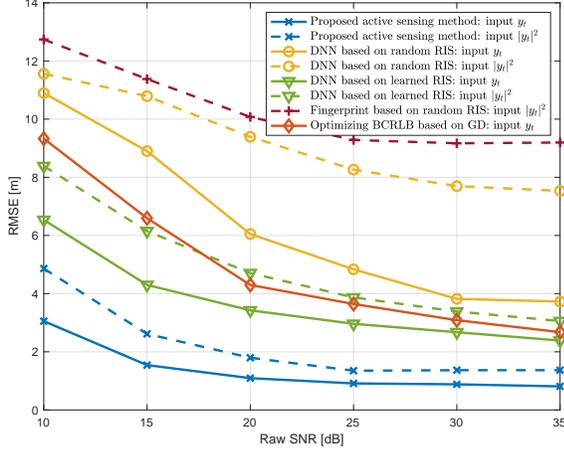
Fig. 3: Localization accuracy vs. raw SNR,  $N = 64$ ,  $T = 6$ .
