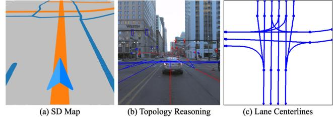
Fig. 1: **Lane-Topology Reasoning.** Leveraging standard definition (SD) map (a) with prior information of the road-level topology, our work aims to improve lane centerline detection (c), lane-topology reasoning between lane centerlines, and traffic elements (b). In the SD map, orange lines and teal lines correspond to roads and pedestrian ways, respectively.
