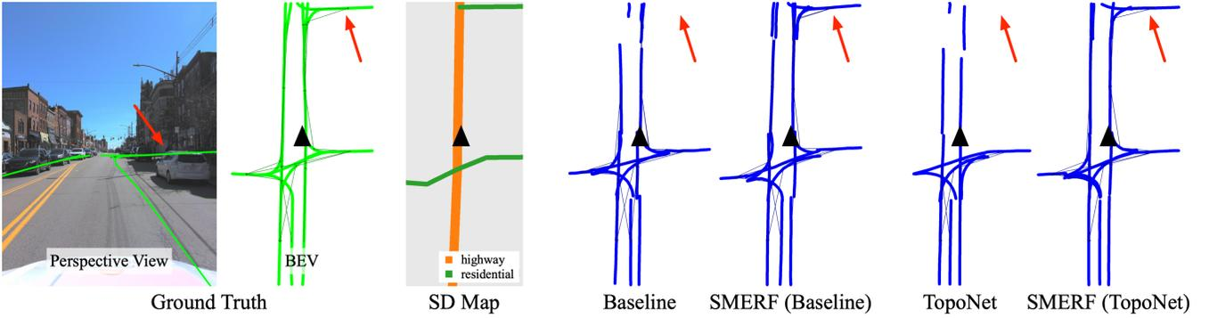
Fig. 4: **Qualitative Results.** We visualize the lane predictions from OpenLane-V2 dataset validation split along with the ground truth lane-topology and the corresponding SD map from the location. Observe that adding SD maps allows the model to infer lanes that are far away and even occluded by a building (marked with the red arrows). We denote the ego-vehicle’s position with a black triangles for visualization purposes.
