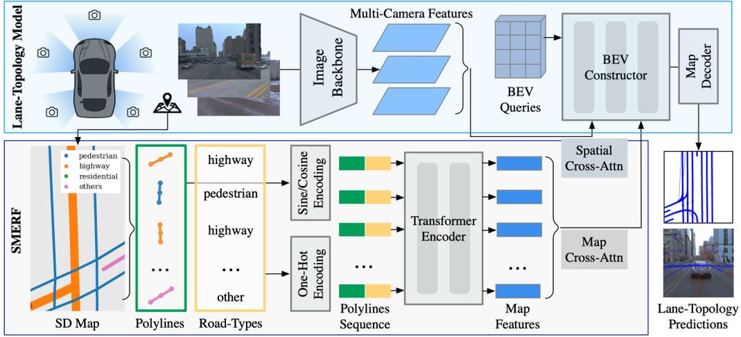
Fig. 2: **Overall approach of SMERF.** The SD map is queried at the ego vehicle’s location as a prior for lane-topology reasoning. SD map is first converted into a polyline-sequence representation, then encoded by a Transformer encoder. Our method is amenable to any transformer-based lane-topology models via cross-attention with the SD map features.
