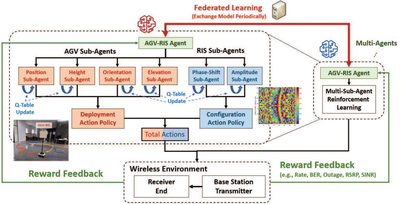
Fig. 2: The proposed federated multi-agent reinforcement learning, including multiple AGV-RIS agents. An AGV-RIS consists of AGV and RIS sub-agents, respectively controlling optimal deployment and RIS configuration. The reward associated with the determined joint action is fed back to the individual AGV-RIS for the next decision. Federated learning is performed periodically, having a longer period than reinforcement learning mechanisms.
