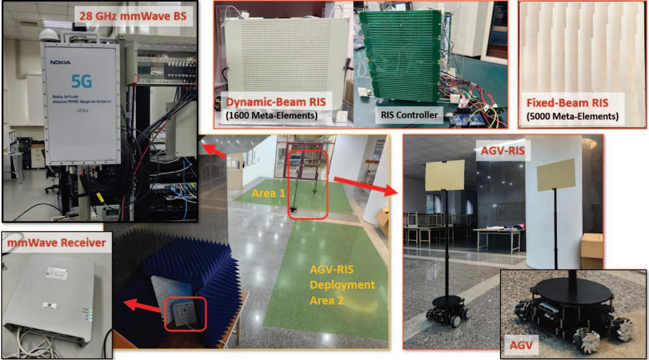
Fig. 1: Prototype of the i-Dris system, including a 28 GHz mmWave BS, an mmWave receiver and AGV-RISs associated with their respective deployment area. There show two types of RISs, i.e., dynamic- and fixed-beam based RISs.
