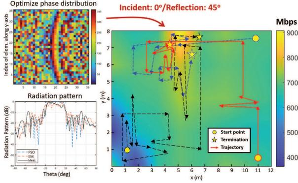
Fig. 3: The trajectory of single AGV-RIS experiments for the proposed i-Driz system. Three start points are evaluated with respect to a place near or faraway from the optimal deployment, and initialization with low-rate region. The rate performance of heatmap are offline collected utilizing exhaustive search. Note that the result is conducted, with the phase-shifts of RIS offline determined.
