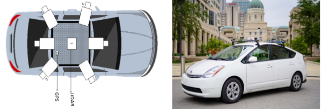
Fig. 11. Overview of the car-based perception system with sensors.
