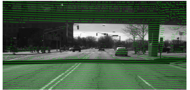
Fig. 1. Example of an accurate LiDAR-Camera mapping result
