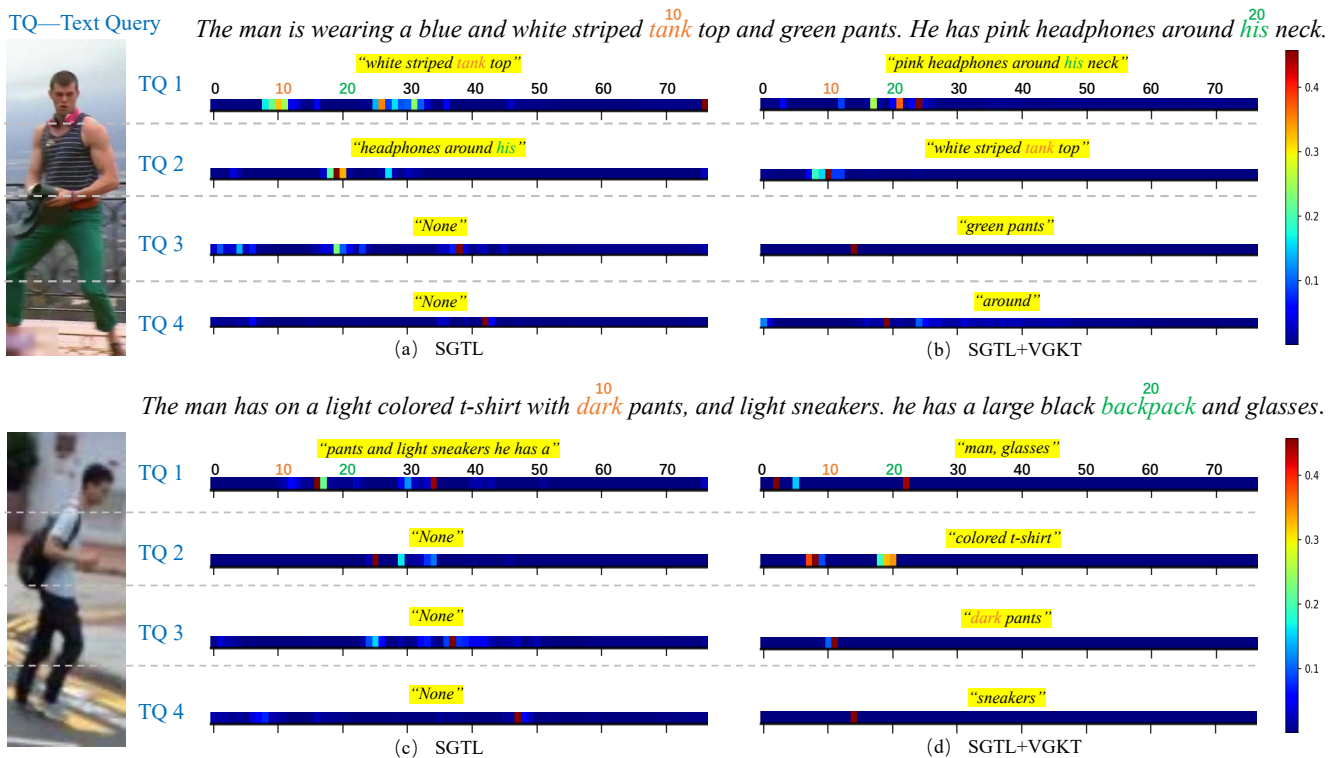
Fig. 6: Visualization of attention maps for four text queries within the SGTL cross-attention block. Each attention map represents the relationship between the i -th text query and the original text description, aiming to estimate its ability to grasp specific fixed-strip body parts. All sentences are standardized to a length of 77 words, with zero padding applied to sentences shorter than 77 words. It is worth noting that the language information corresponding to zero padding is denoted as “None”. For ease of comprehension, we have highlighted the 10-th word in orange and the 20-th word in green. Additionally, words with significant attention weight are denoted with a yellow background color. Different colors represent different attention scores. Please refer to the colormap on the right for the correspondence between colors and attention values.
