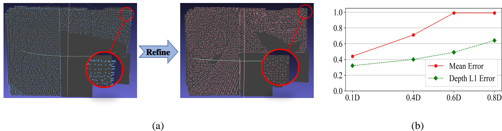
Figure 8: Map Refinement and Sampling Concentration Ablation. (a) From a bottom view of Apartment-1, we can observe that there is an offset in the unrefined neural point cloud (blue), while the refined neural point cloud (pink) fits well. (b) As the sampling points diverge, the error rises.
