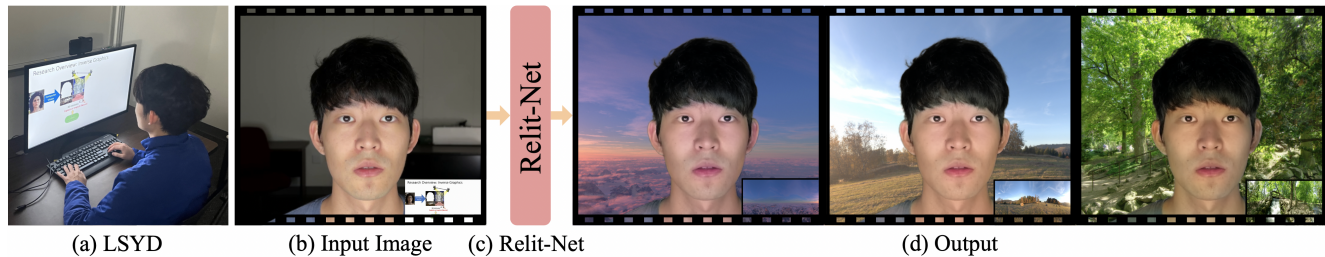
Figure 1. We use our Light Stage at Your Desk (LSYD) dataset to build a personalized relighting algorithm that generates temporally consistent and high-quality portrait videos under different lighting conditions. This data could easily be captured at home, as it just consists of recordings of users while watching videos at a monitor. We used background matting [16] to replace the original background with a portion of the environment map.
