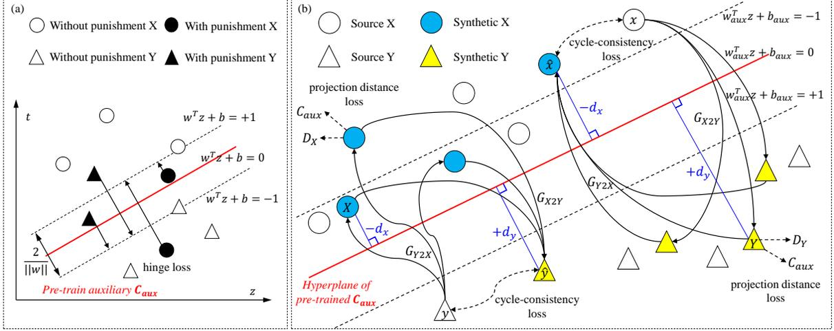
**Fig. 1.** Overview of ParaGAN enabling cyclic parameterized projection. (a) Pre-train an auxiliary classifier  $C_{aux}$  by hinge loss to provide a hyperplane. (b) The generators translate source images conditioned on the target images' projection distances in forward path, and vice versa for reconstructing sources.  $C_{aux}$  reconstructs the projection distances from synthetic images.
