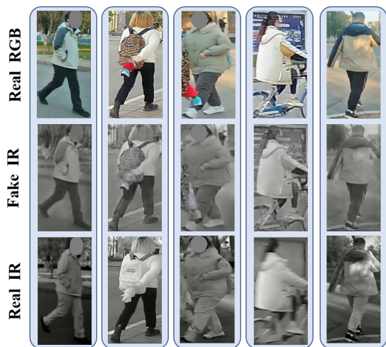
Fig. 7. Visualization of sampled real RGB, generated fake IR and real IR images. Same ID for the same column.
