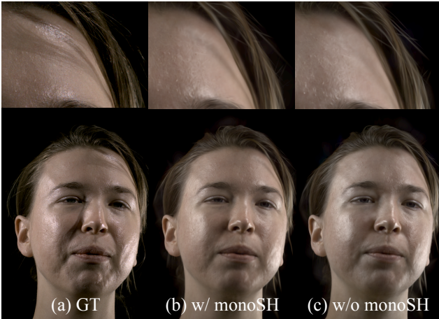
Figure 6. Ablation Study: Monochrome SH. Compared to a held out frame (a), using higher-order monochrome SH coefficients (b) improves the sharpness of shadows compared to a model without them (c).
