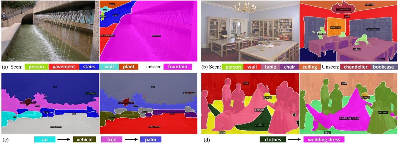
Figure 6. Visualization segmentation results of our SCAN. The correspondence between categories and colours is shown below each image for clear. (a) and (b) demonstrate the excellent segmentation of our method for seen and unseen categories. (c) and (d) displays the adaptability for flexible text query. Best viewed in color.
