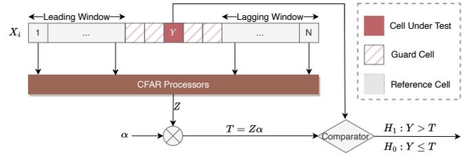
Fig. 5. Overview of CFAR processing. Set of  $X_1, X_2, \dots, X_N$  represents the detection window,  $Y$  is the value of CUT,  $Z$  represents the clutter background level of the CUT,  $T$  is the detection threshold,  $\alpha$  donates a scaling factor,  $H_1$  declares that an object is located within the CUT,  $H_0$  indicates that there is no object in the current CUT.
