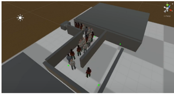
(a) Simulation of Queue Scene 3 considering MarkerDensity = 0.75 , AgentRadius = 1 , and a wide space between obstacles.
