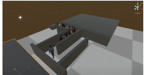
(b) Simulation of Queue Scene 2 considering MarkerDensity = 0.75 , AgentRadius = 1 , and a narrow space between obstacles.
