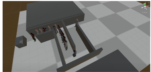
(d) Simulation of Queue Scene 2 considering MarkerDensity = 0.5 , AgentRadius = 5 , and a narrow space between obstacles.
