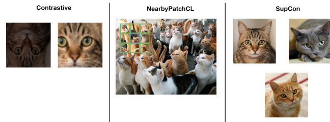
Fig. 1. In contrastive learning [8], our NearbyPatchCL, and SupCon [16], positive samples are handled differently. Contrastive learning involves augmented pairs from the same image. In SupCon, it includes all images with the same label, while NearbyPatchCL defines positive samples that encompass all views of the center patch (blue border) and nearby patches (green border).
