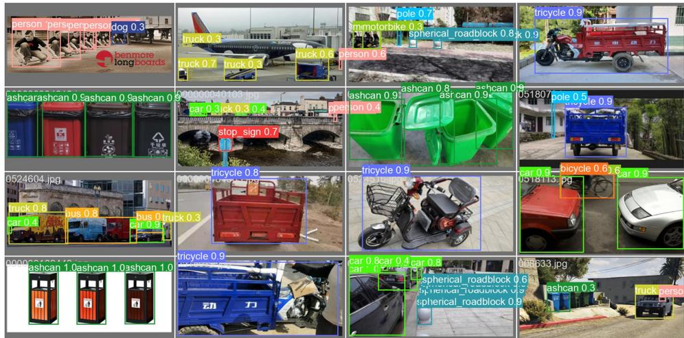
**Fig. 5** Visualization of the performance of YOLOv8 with bounding boxes and corresponding obstacle classes predicted by the model along with the respective confidence scores
