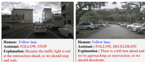
Figure 5. The zero-shot performance of DriveMLM on the real driving scene from nuScenes dataset. (a) DriveMLM can recognize the red light and stop (b) DriveMLM can infer the location of the intersection and slow down in advance.
