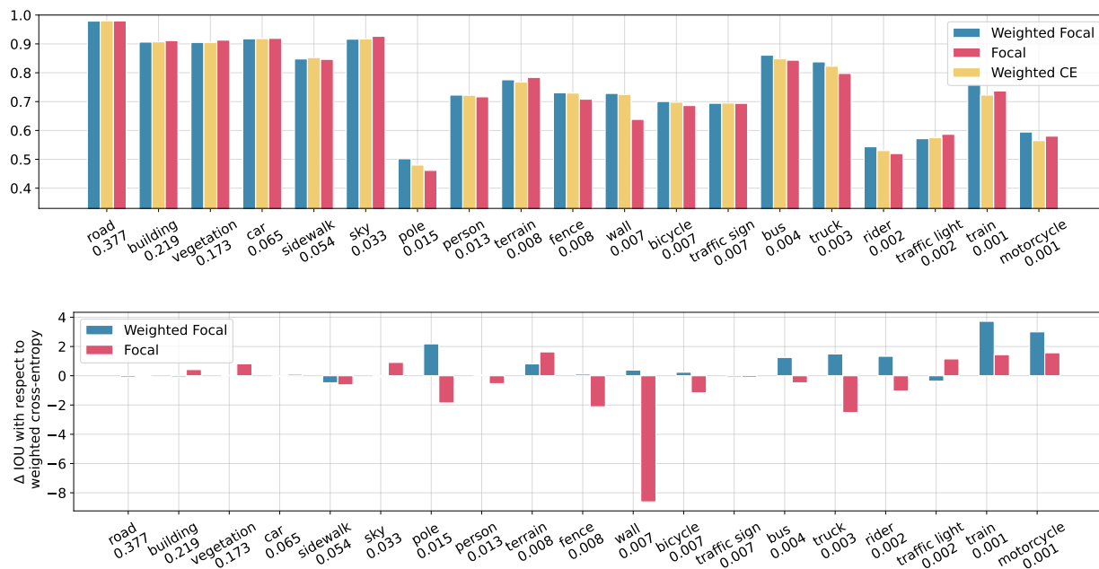
Figure S5 Top: Per-class IOU MF on Cityscapes with models trained with different loss functions using ConvNext-L backbone. Labels are sorted according to their frequency in the validation images, which is written below the class name. Bottom: Per-class difference in IOU MF of models trained with weighted and non-weighted focal loss w.r.t. the model trained with weighted cross-entropy (CE) loss. (Best viewed in color.)
