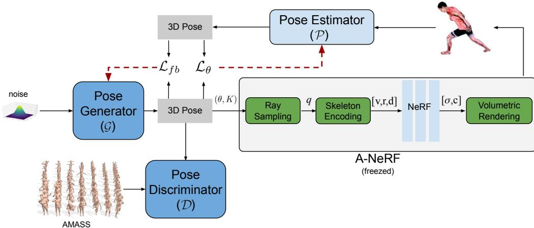
Figure 2: The overall framework of the proposed *PoseGen*. The pose generator learns to generate input of novel poses  $\theta$  and camera viewpoints  $K$  which are fed to a NeRF model to render human images. The 3D pose estimator is trained with rendered images and provides feedback to the pose generator. The feedback function enforces the generator to generate OOD data.
