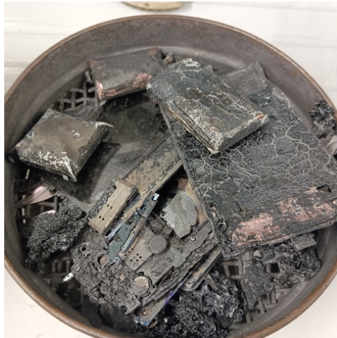
Figure 1: Pyrolyzed smartphones for battery separation.
