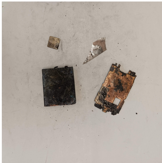
Figure 3: Sample image of components on a white background. The components are samples of glass, PCB, battery, and metal piece, from the top right on, clockwise.
