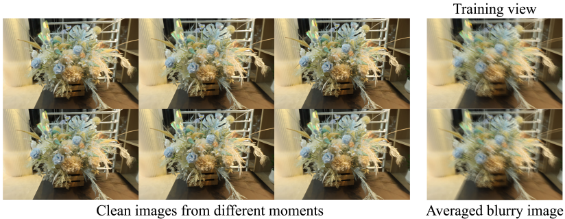
Fig. 6: Camera motion blur modeling during training. Clean images at different moments of the camera movement during exposure time are rasterized and averaged to a single image to model the camera motion blur.
