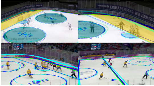
Figure 15. Example results on Olympic validation data. Light blue is initial homography estimate, dark blue is the final homography after refinement, and green indicates ground truth. These cases show that although the alignment can be quite close usually, sometimes the alignment can still be off even after refinement for the Olympic rinks, likely due to the difficulty in segmenting these rinks.
