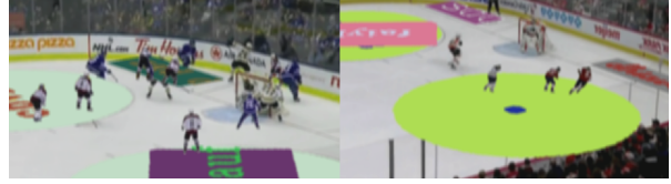
Figure 5. Examples of logo augmentation, which sometimes added text, rectangles, and circle fillings in order to augment the existing dataset further.
