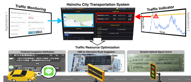
Figure 5: System integration of GCT flow enables real-time crowd monitoring and threshold alerts. Exceeding city-defined limits triggers traffic optimization strategies.
