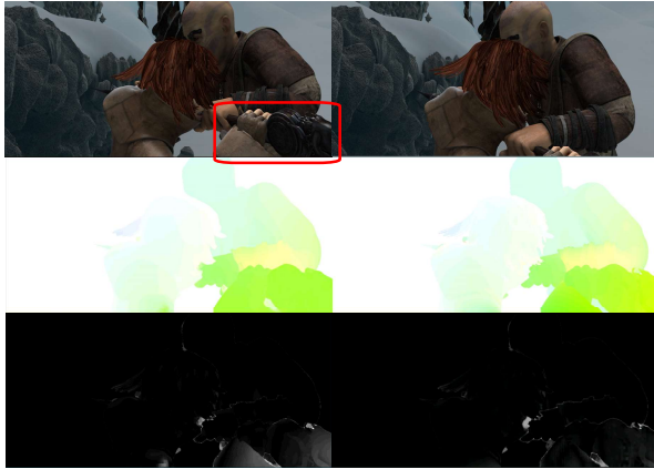
Figure 6: The first row is the frame pair, the second row from left to right is the optical flow output from GMFlow and YOIO respectively, and the third row is the EPE map corresponding to the optical flow of the previous row. In the EPE map, the brighter the color, the greater the error.
