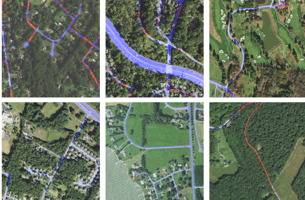
Fig. 2. Example images and labels from the proposed Chesapeake Roads Spatial Context (RSC) dataset. Labels are shown over the corresponding NAIP aerial imagery with the “Road” class colored in blue and the “Tree Canopy over Road” class in red.
