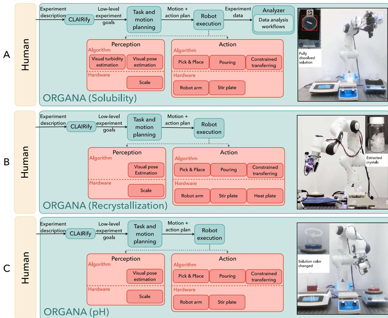
Fig. 4: **Instances of ORGANA conducting various chemistry experiments.** A) solubility, B) recrystallization, C) pH testing. Snapshots depict the robot executing actions in each setup, alongside images of the end results.
