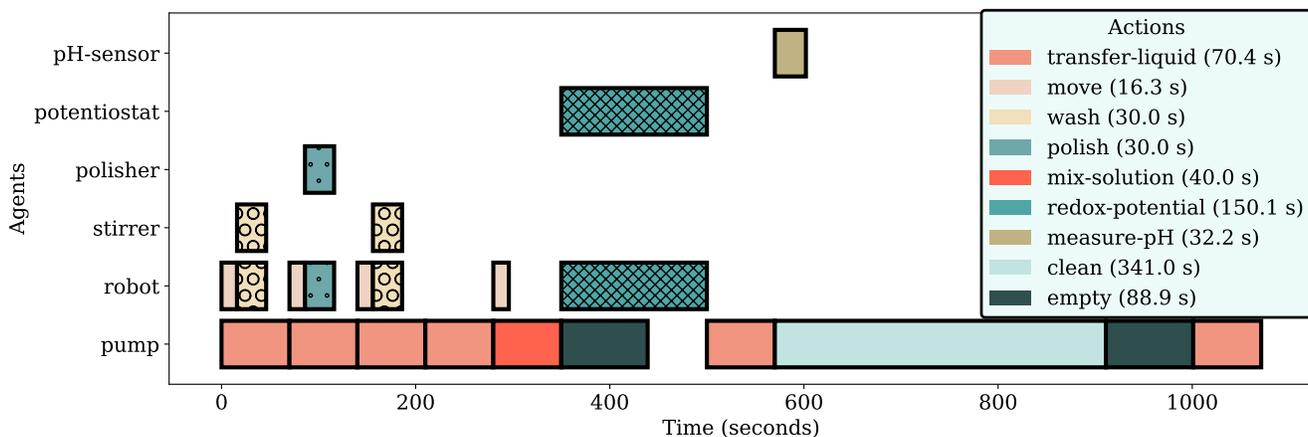
Fig. 7: **Gantt chart of electrochemistry experiment with parallel execution.** The execution times are written in the legend. Note: pump cannot transfer solution to pH beaker at  $\sim 500$  sec due to ongoing redox potential measurement. Boxes stacked on top of each other with the same color and pattern mean that the agents are involved in performing the same action jointly.
