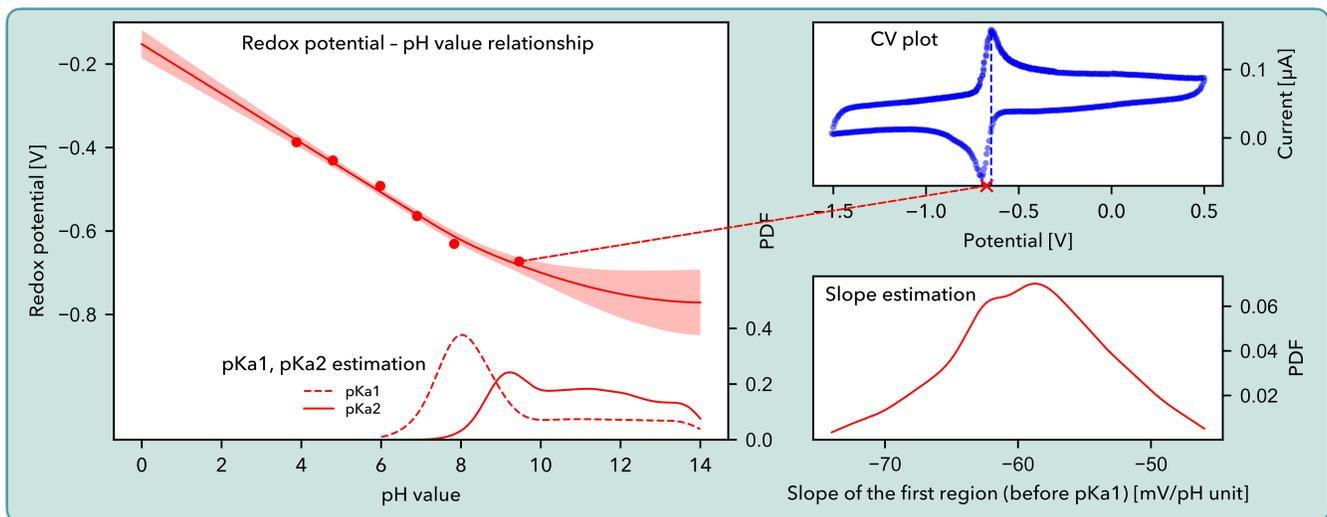
Fig. 6: **The electrochemistry results executed by ORGANA.** On the left, a Pourbaix diagram is shown for a single ORGANA experimental run with estimated distributions for  $pK_{a1}$  and  $pK_{a2}$ . Maximum likelihood estimation (MLE) for  $pK_{a1}$  is 7.86. In the top right, cyclic voltammetry for  $pH=9$  is depicted. In the bottom right, estimated distribution of the slope for the first region is shown, with an MLE of  $-61.8$  mV/pH unit.
