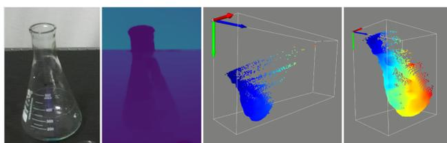
Fig. 13: **Visualizations of the RGBD image and 3D point clouds for an Erlenmeyer flask.** the two figures on the right display the point cloud generated from the raw sensor depth map, and the point clouds after outlier removal.
