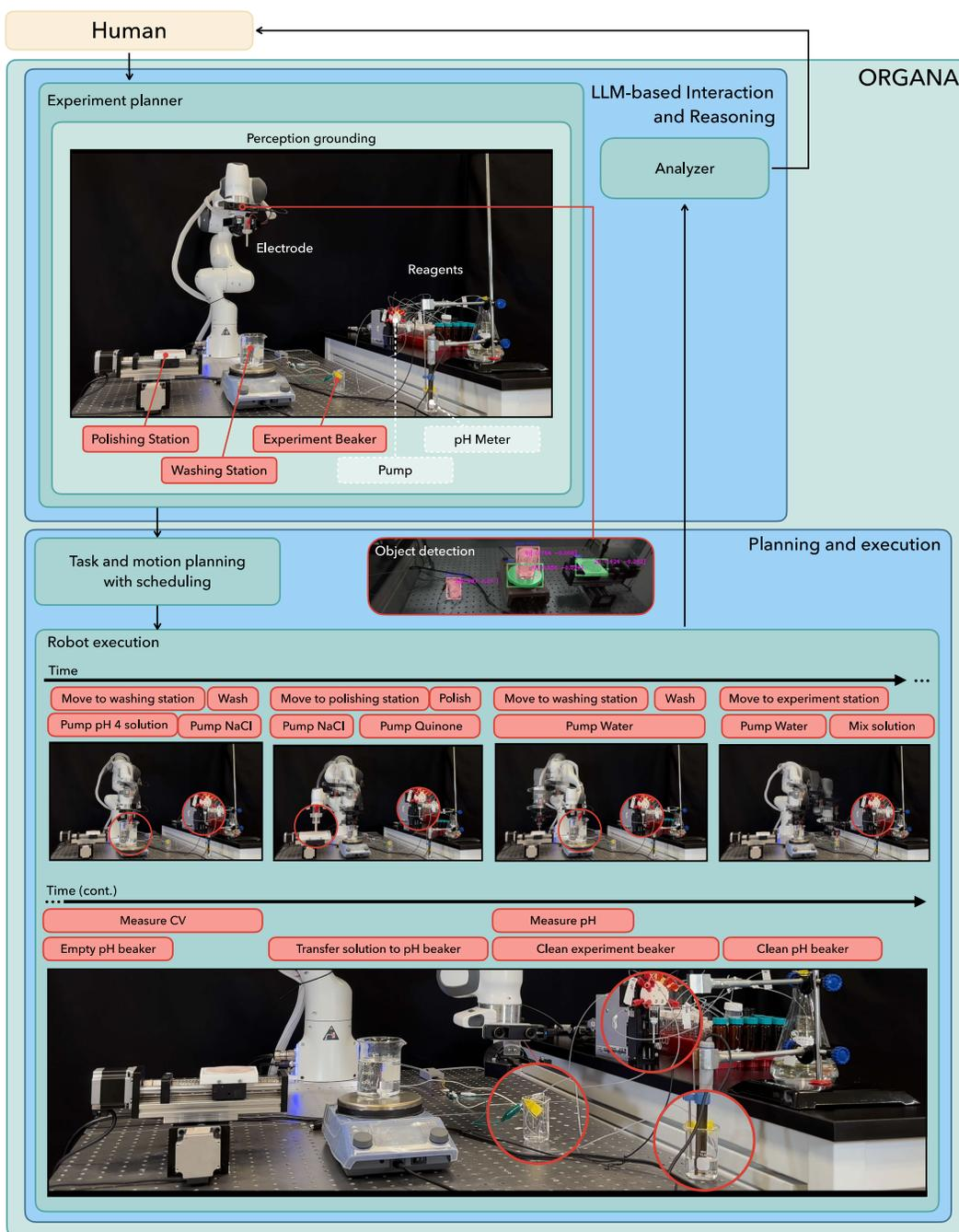
Fig. 5: **The electrochemistry setup and experiment workflow.** Initially, users communicate their intention to ORGANA; objects and their poses are perceived. Subsequently, the user interacts with ORGANA to establish object functionalities. Eventually, ORGANA plans the robot actions for parallel execution. On top, it shows the experiment setup. At the bottom, it displays the results of visual perception and snapshots of the robot and other hardware executing the actions in parallel.
