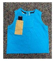
Fig. 2. Child vest with Sony recorder (1.43"\*4.31"\*6.13") in the front pocket.
