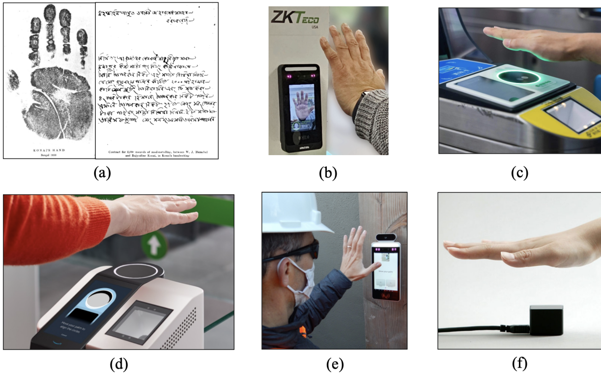
Fig. 1: Applications of palmprint recognition; (a) The earliest use of a palmprint impression by Sir William Herschel as a signature for a contract [5] in the 1850s, (b) mobile contactless palmprint recognition system by ZKTeco/Armatura [6], (c) contactless palmprint recognition for train and metro systems in China by Tencent [7], (d) Amazon One system for seamless and unattended grocery shopping [8], (e) contactless palmprint recognition system by RedRock for employee attendance [9], and (f) PalmSecure palm vein recognition by Fujitsu Global [10].
