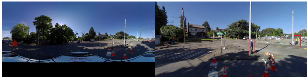
Fig 1. Sample images from the pedestrian detection data pipeline. The left image is an original 360° image from a data collection run. The image on the right is the right-hand side of the original image after orthorectification and pedestrian detection (both sides of the image are processed separately). There are two pedestrians that were detected by the algorithm (in red bounding boxes).
