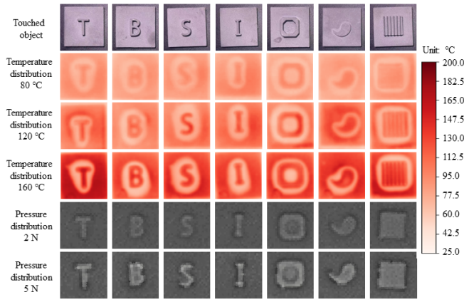
Fig. 6. SATac touches different objects for testing their properties, and obtains corresponding temperature distribution (80 °C, 120 °C, and 160 °C) and pressure distribution (2 N and 5 N).
