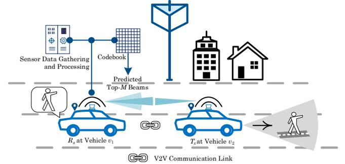
Fig. 1: Illustration of considered mmWave enabled V2V communications system model.
