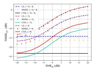
Fig. 13: NMSE<sub>UE</sub> vs SNR<sub>SI</sub> for different pilot dimensions, SNR<sub>UE</sub> = 5 dB.
