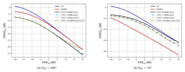
Fig. 8: NMSE<sub>SI</sub> vs SNR<sub>SI</sub> for (a) low-correlated and (b) high-correlated channels.
