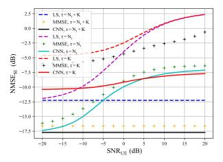
Fig. 11: NMSE<sub>SI</sub> vs  $SNR_{UE}$  for different pilot dimensions,  $SNR_{SI} = 0$  dB.
