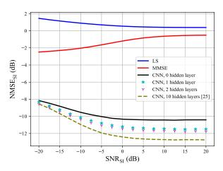
Fig. 6:  $NMSE_{SI}$  vs  $SNR_{SI}$  with a varying number of hidden layers for a full-duplex BS with 1-bit ADCs.
