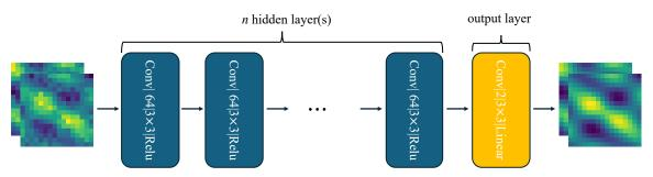
Fig. 3: The CNN architecture employed for SI and UE channel estimation. we apply n (n = 0, 1, 2, 10) convolutional hidden layer(s) each with a  $3 \times 3$  window size and 64 convolutional kernels.
