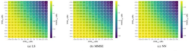
Fig. 14: NMSE<sub>UE</sub> vs SNR<sub>SI</sub> and SNR<sub>UE</sub> for (a) LS and (b) MMSE (c) NN channel estimators,  $\tau = K$ .
