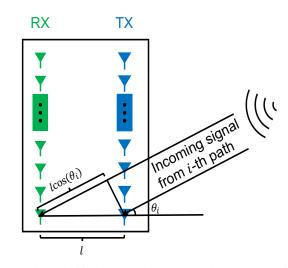
Fig. 4: Phase shift between the RX and TX arrays in the separate antenna configuration in a full-duplex BS.
