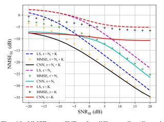
Fig. 10:  $\text{NMSE}_{SI}$  vs  $\text{SNR}_{SI}$  for different pilot dimensions,  $\text{SNR}_{UE} = 0$  dB.
