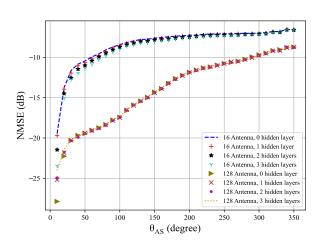
Fig. 16: NMSE of channel mapping between RX and TX arrays vs angular spread.
