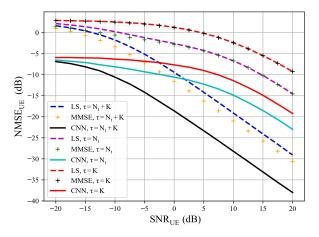
Fig. 12:  $\text{NMSE}_{\text{UE}}$  vs  $\text{SNR}_{\text{UE}}$  for different pilot dimensions,  $\text{SNR}_{\text{SI}} = 10 \text{ dB}$ .
