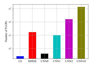
Fig. 18: Number of FLOPs for SI channel estimation of different estimators. CNNx represents a CNN with x hidden layer(s).
