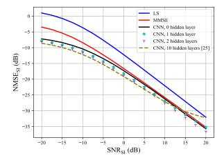
Fig. 5:  $NMSE_{SI}$  vs  $SNR_{SI}$  with a varying number of hidden layers.
