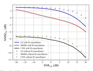
Fig. 15: UE channel estimation with/without SI cancellation,  $\tau = K$ , SNR<sub>SI</sub> = 20 dB.
