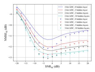
Fig. 7:  $NMSE_{SI}$  vs  $SNR_{SI}$  with a varying number of hidden layers for a full-duplex BS with few-bit ADCs.
