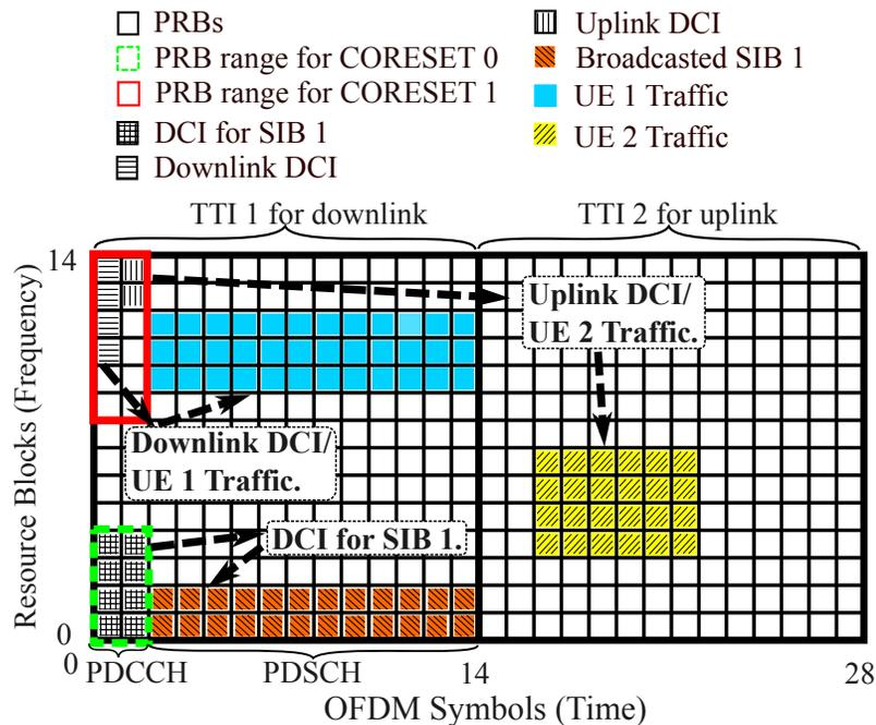
**Fig. 6**— An overview of DCI and data transmission in the 5G physical layer. There are multiple CORESETs, each of which occupies part of the bandwidth, and the DCIs point to the resource blocks that UE should receive from or send data to.
