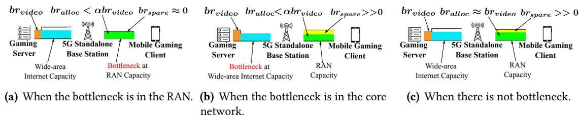
Fig. 4— The possible situations with bottleneck in different position of the network.
