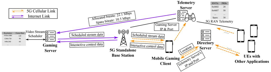
**Fig. 1— TGaming: System Overview.** TGaming’s **Cloud Gaming Server** receives exact capacity estimates of the 5G Standalone Radio Access Network from TGaming’s **5G Standalone Telemetry Server**, thus adjusting its video resolution and frame rate to accommodate the RAN’s capacity. While the scope of this paper is mobile cloud gaming, our telemetry tool is general, estimating spare capacity for any end-to-end transport protocol or application.
