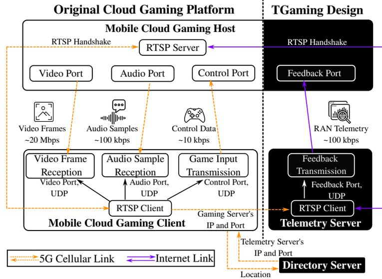
Fig. 2— Overview of TGaming’s overall architecture.<sup>1</sup>
