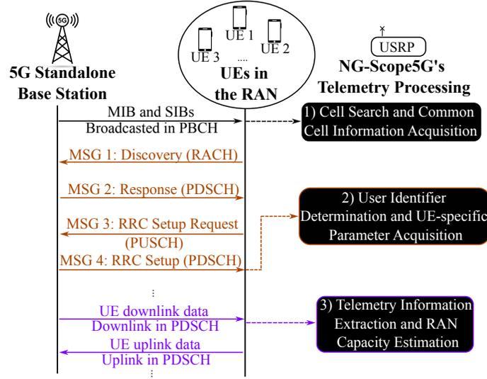
**Fig. 5—** *NG-Scope5G telemetry design overview:* NG-Scope5G passively listens to raw radio data and decodes radio resource control messages and DCIs from it. NG-Scope5G’s processing components are denoted by a black background.
