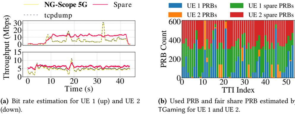
**Fig. 14**— NG-Scope5G telemetry example trace: We calculate the bit rate over time. Then we split the free PRBs equally among UEs and use the same parameters in used PRBs to calculate the bit rate provide by the free PRBs.
