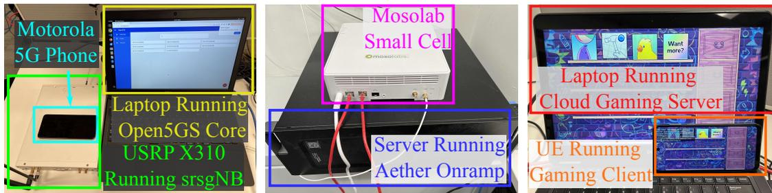
Fig. 7— Hardware used in the TGaming implementation.
