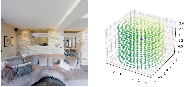
Fig. 1. Example of simulated environment (left) and cylindrical grid used for sound positioning (right).
