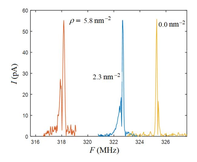
FIG. 6. Determination of helium coverage on the suspended carbon nanotube at 0.25 K. The shift of the resonance is due to increase in the mass of the oscillating nanotube, while the additional stiffness can be ignored because helium is in a fluid phase.
