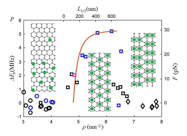
FIG. 1. Resonance frequency shift  $\Delta F_0$  due to 1D pressure (force) of zero-point phonons (T < 20 mK) as a function of atomic coverage per nm<sup>2</sup> (lower axis) and the corresponding length occupied by the 1/3 solid,  $L_{1/3} = L(\rho - \rho_L)/(\rho_{1/3} - \rho_L)$  (higher axis). Curve displays the contribution of the Casimir force,  $\mathcal{F}_{\rm C} = 50\hbar c \pi \mathcal{L}/L^3$ , see text for details.
