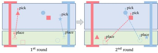
(a) Unwise assignment: motion interference exists in the 2<sup>nd</sup> round
