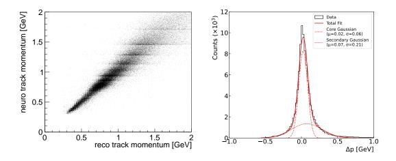
Figure 13: Left: Correlation of the true track momentum from reconstructed tracks and the momentum estimated for the neural tracks. Right: Difference of track momenta (see text).
