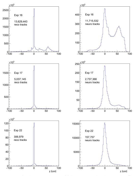
Figure 9: Left column: Distributions of fully reconstructed tracks using the offline reconstruction software package. Right column: Distributions of found neural tracks. Upper row: Exp. 16, the neural z-trigger was not yet enabled. Middle row: Exp. 17 with z-trigger enabled for this and the following experiments. Lower row: Exp. 22 (end of 2021 running). In this latter period the machine background was significantly reduced (see text).
