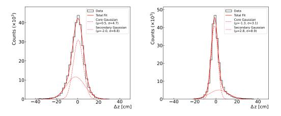
Figure 10: Difference of the z-positions between the reco track and the associated neuro track, in [cm], for Exp. 16 (initial FANN training) and Exp. 24 (presently used Pytorch training). The distributions are fitted with double Gaussians (see text).
