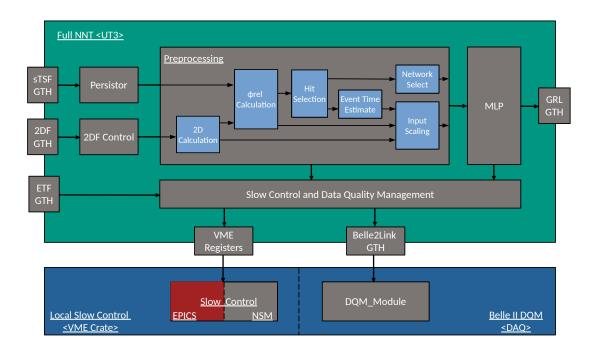
Figure 7: Details of the overall architecture of the neural trigger hardware.
