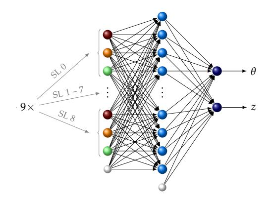
Figure 5: Sketch of chosen architecture for the fully connected feed-forward neural network. The input consists of 9 triplets of data from the 9 SLs, giving a total of 27 inputs. Due to limitations in the latency only 81 nodes in a single hidden layer are implemented. Two output nodes provide the estimates for the z origin of the track and its polar emission angle  $\theta$ .
