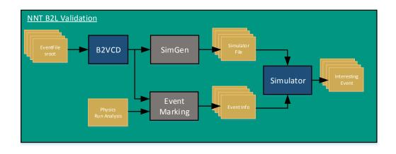
Figure 8: Process for offline verification of the hardware on clock cycle granularity.
