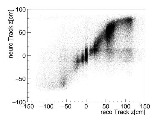
Figure 15: Correlation of the z-impact between the fully reconstructed tracks and the corresponding neuro tracks. The horizontal band between  $\pm$  15 cm marks the acceptance region of the single track trigger. The "feed-down" effect into this band, mainly from the z intervals  $\pm$  20 cm and  $\pm$  50 cm, is clearly visible. The data were taken in a short run where the z-Trigger was not enabled.
