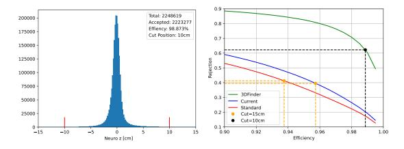
Figure 16: Expected performance of a deep-learning network architecture with 3D track candidates as input plus topological information from all wires in the associated track segments ("3DFinder"). Left: z estimate of the 3DFinder network for IP tracks, right: rejection of background vs. efficiency for IP tracks, green curve), compared to the present networks in blue and red (see text).
