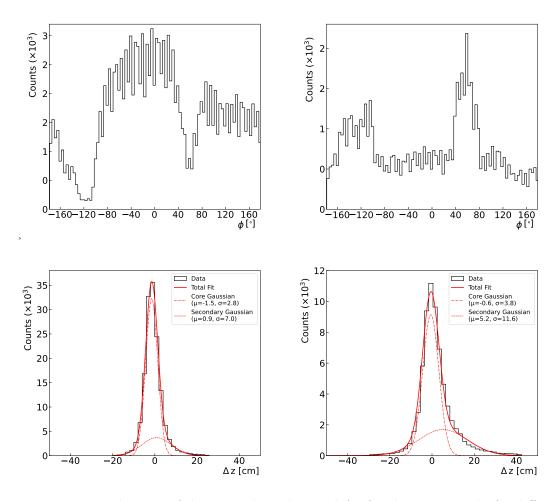
Figure 11: Distributions of the azimuth angle  $\phi$  and  $\Delta z$  for the neuro tracks for different numbers stereo SLs. Left column: neuro tracks with all 4 SLs. right column: neuro tracks with one of the stereo SLs missing. Data from early 2022 running (Exp. 24). For about 70% of the tracks signals from all stereo Sls were present in this experiment.
