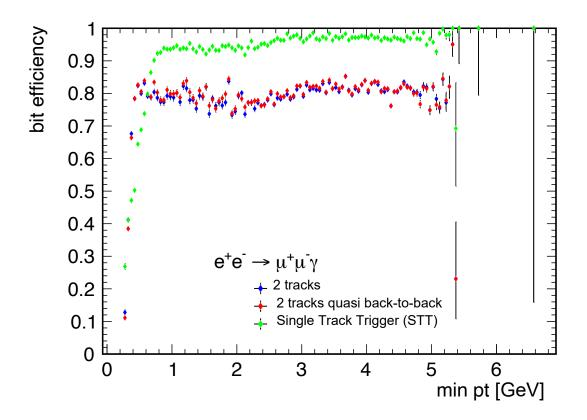
Figure 14: Efficiency of STT in comparison to the two-track triggers for the reaction  $e^+e^- \rightarrow \mu^+\mu^-(\gamma)$ , as function of the smaller transverse momentum of the two tracks.
