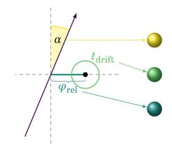
Figure 4: Preprocessing of input variables to the neural network: for each TS contributing to a neural track, a triplet of variables is prepared, which give the crossing angle  $\alpha$  of the track candidate through the TS, the angle  $\varphi_{rel}$  of the priority wire, and the signed drift time (see text).
