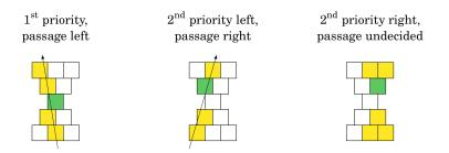
Figure 3: Examples of hit patterns (in yellow) with different priority cells and left/right state. The priority cell in each of the three examples is shown in green. In the case of undecided left/right passage, such as on the rightmost pattern, the drift time is set to 0, irrespective of the transmitted drift time.
