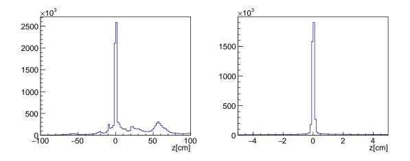
Figure 1: Left: Distribution of the z-positions in centimeters of reconstructed tracks from Belle II, over the entire z range. Right: same as left, but with higher resolution in z around the IP. The events from  $e^+e^-$  collisions contribute only about 20% of all events. The data is from the running in the year 2020, before the launch of the z-Trigger.
