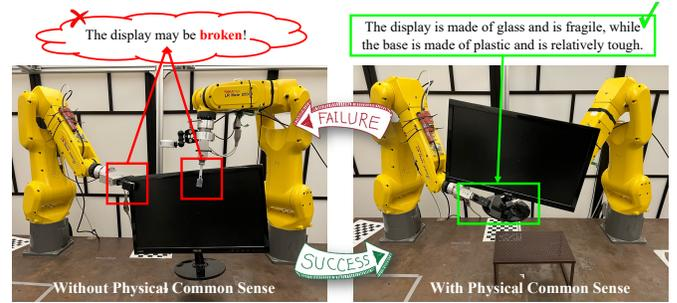
Fig. 1: Motivation of PhyGrasp. Current robot grasping policies (left) typically predict grasping poses based solely on the object’s 3D shape, neglecting its physical properties. This oversight can lead to potential damage to the display. In contrast, integrating physical common sense into robotic systems (right) can address this issue effectively.
