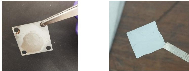
Figure 12: Cd deposited on Cu backing and Cd deposited on Mylar backing targets
