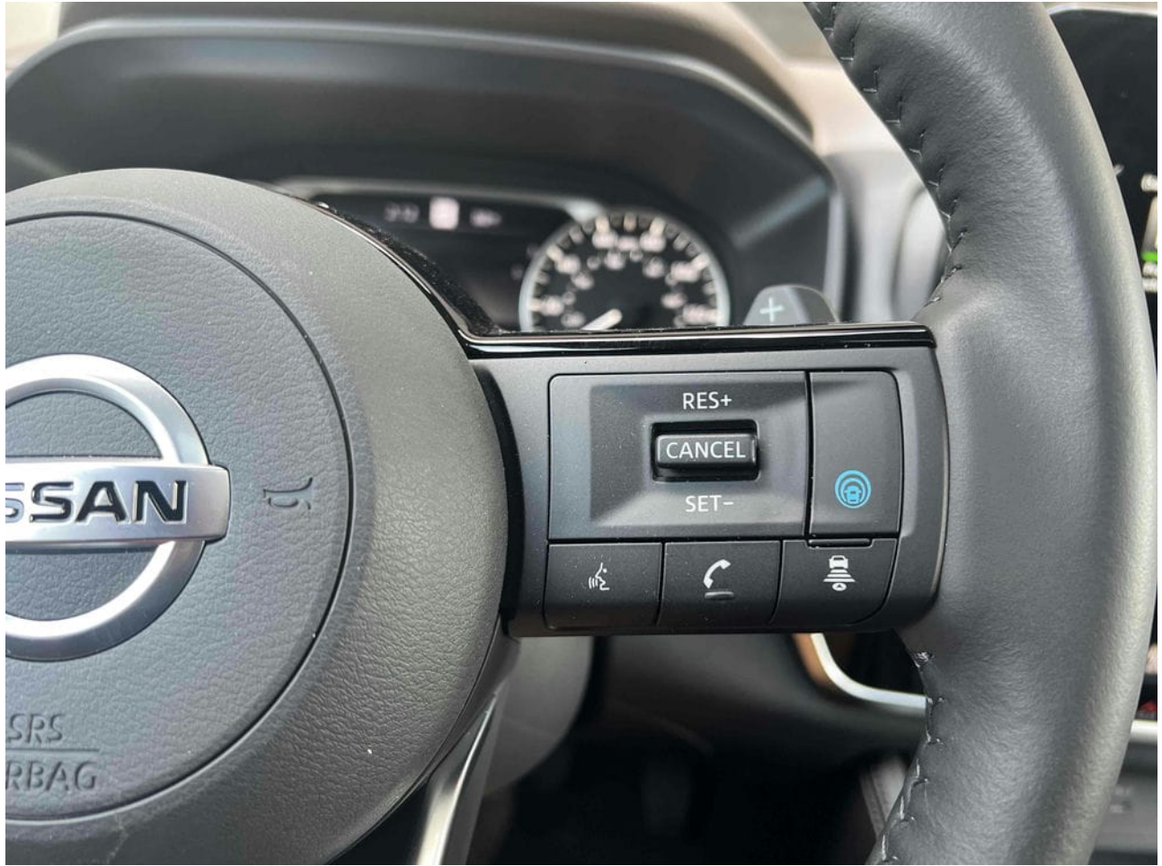
FIGURE 7 A photograph of a Nissan Rogue’s steering wheel buttons that control the vehicle’s ACC. The ACC system is turned on by manually pressing the blue icon on the far right. Through our vehicle interfacing efforts, we are able to electronically press the + and – buttons to toggle the ACC speed setting up 1 mph and down 1 mph, respectively, or hold them to increment by 5 mph. The three ACC gap settings are rotated through by pressing the button on the bottom right.
