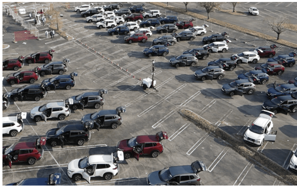
FIGURE 15 A WiFi antenna is placed in the center of the vehicle parking lot, enabling OTA data uploads and software updates for each Raspberry Pi in each vehicle.
