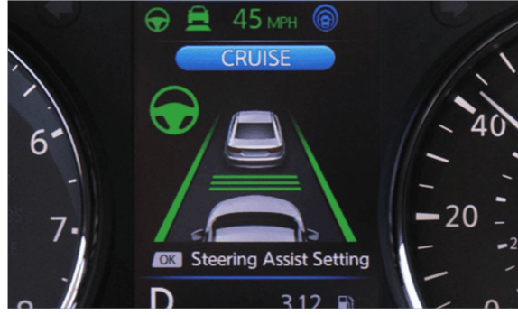
FIGURE 25 Dashboard view while the RL controller is being run. The speed setting is set at 45 MPH and the gap setting is set at three bars.
