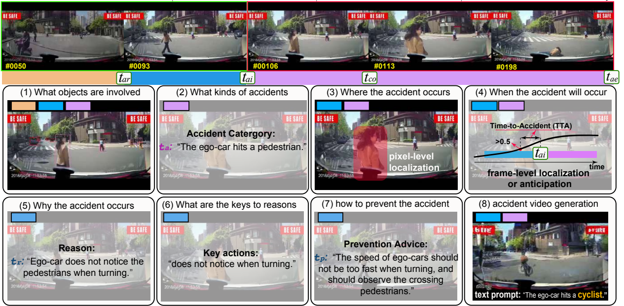
Figure 1. The ego-view multimodality accident video understanding tasks that MM-AU can support, where we highlight the text descriptions for accident reason ( t_r ), prevention advice ( t_p ), and accident category ( t_a ), as well as temporal windows (accident-free ■ , near-accident ■ , and accident ■ windows) for different tasks.
