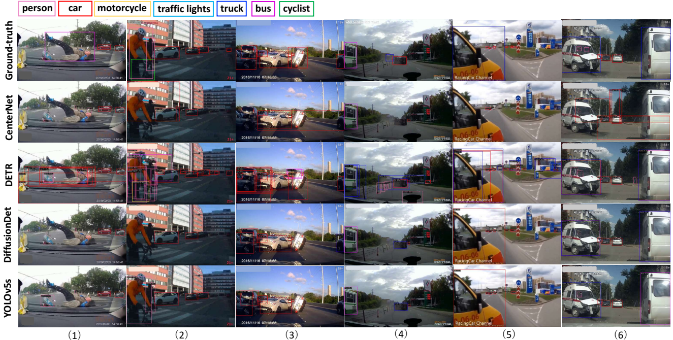
Figure 2. The object detection snapshots in accident frames by CenterNet [30], DETR [4], DiffusionDet [7], and YOLOv5s [23]. We can see that all detectors fail to detect the cyclist (column (2)) and the pedestrian with distorted posture (column (1)). DETR is more active for covering all possible objects while many false detections are generated.
