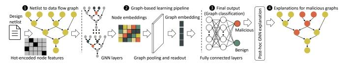
Fig. 4. Proposed MaliGNNoma methodology: Synthesized netlists are transformed into DFGs for training a GNN to separate malicious and benign samples. A GNN explanation tool identifies nodes contributing to malicious classification.
