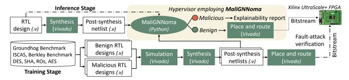
Fig. 7. MaliGNNoma experimental setup and tool flow.
