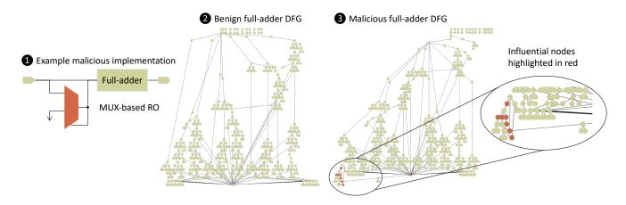
Fig. 5. Example of malicious full-adder with a MUX-based RO connected to its input. 2 The DFG of a benign full-adder without the MUX-based RO. The DFG with the MUX-based RO included. Also illustrates the output of the GNN explainer, highlighting the malicious nodes in the DFG, which correspond to the MUX-based RO.
