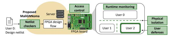
Fig. 3. Multi-tiered defense system for securing cloud FPGAs. Defense mechanisms, highlighted in green, include netlist checking, access control, physical isolation, and runtime monitoring implemented by the CSP. Users can further enhance security with design-level defenses such as masking and active measures.
