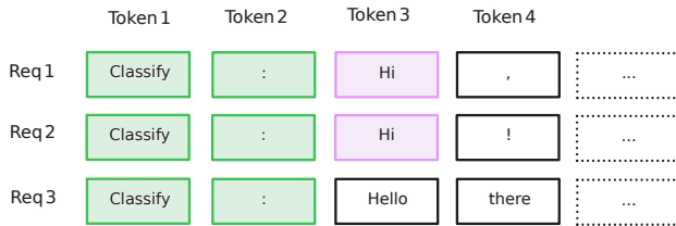
Figure 1: Example of prefix sharing across requests in a KV cache. Green tokens (“Classify” and “:”) are universally shared across all three requests. This means that only one set of KV needs to be computed, reducing redundant computations. Purple tokens (“Hi”) represent partial sharing between Req 1 and 2, illustrating selective reuse. Black tokens are the ones that require computation.
